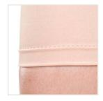
Ultrasonic technology enables joining of textiles by welding. Finishing with this technology is very durable and the fabric is less prone to tear.
